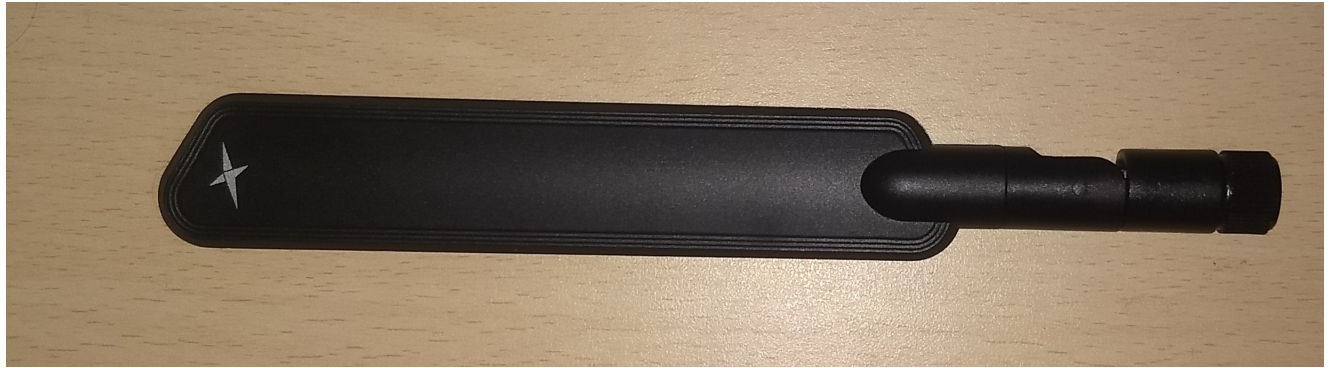
Figure 9: Antenna (TG.55.8113) used to transmit at 3.5 GHz
